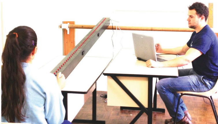
Figure 1 — The Bassin anticipation timer apparatus (Model 35575, from Lafayette Instruments, Lafayette, IN) and the experimental setup.
